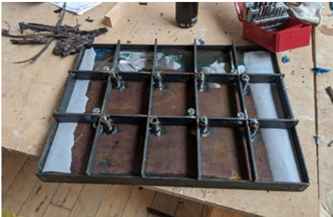
Example of jig used for applying compression on plastic at predetermined positions.
