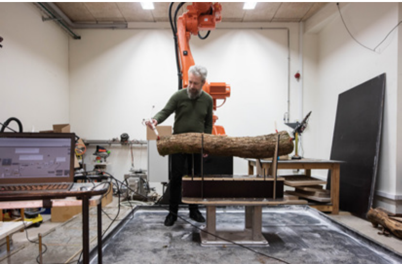
An OptiTrack system is used to locate the marked points on the surface of the log and match them with the 3D model of the trunk.
