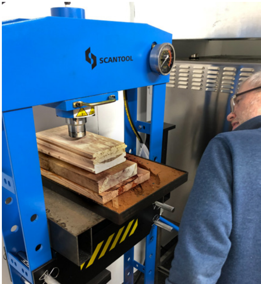
The heated plastic in metal jigs is placed in a press during cooling. The press has also been used in later studies using casting sand to form new plastic building components.
