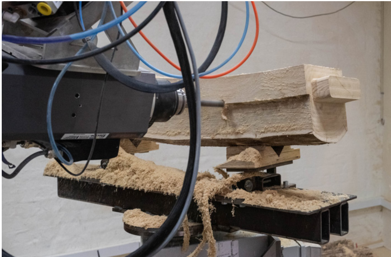
CNC cutting of a trunk where a spindle is mounted on a robot arm. Using an automatic rotary table, it was possible to cut three sides of the trunk as well as the details of the joint without needing to move the trunk.
